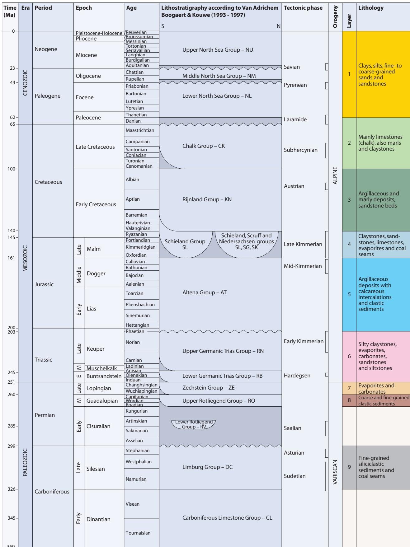
*Fig. 1. Geologic time scale (after Gradstein et al. 2004), lithostratigraphic column (after Van Adrichem Boogaert and Kouwe, 1993 - 1997), main tectonic deformation phases and lithostratigraphic layers at the basis of VELMOD-1 with their lithologic characteristics.*
