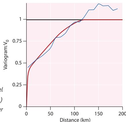
Fig. 11. Variogram model of  $V_0$ -data (VELMOD-1) for the Lower and Upper Germanic Trias groups.
