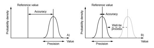
Figure 1 A) Accuracy is the proximity of measurement results to the true value; precision, the repeatability, or reproducibility of the measurement. B) Combined accuracy-precision workflow applied to DGM-deep.
